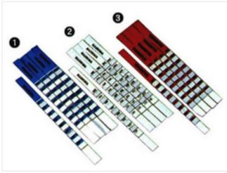
To check the temperature accuracy of fusing presses and irons, thermo paper is used.
